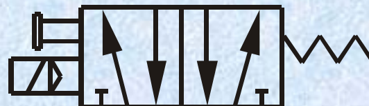
4 way, 5 port, 2 position solenoid operated with manual over ride
